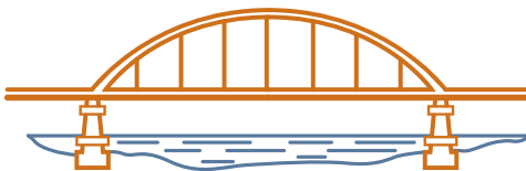
Tied Arch Bridge
